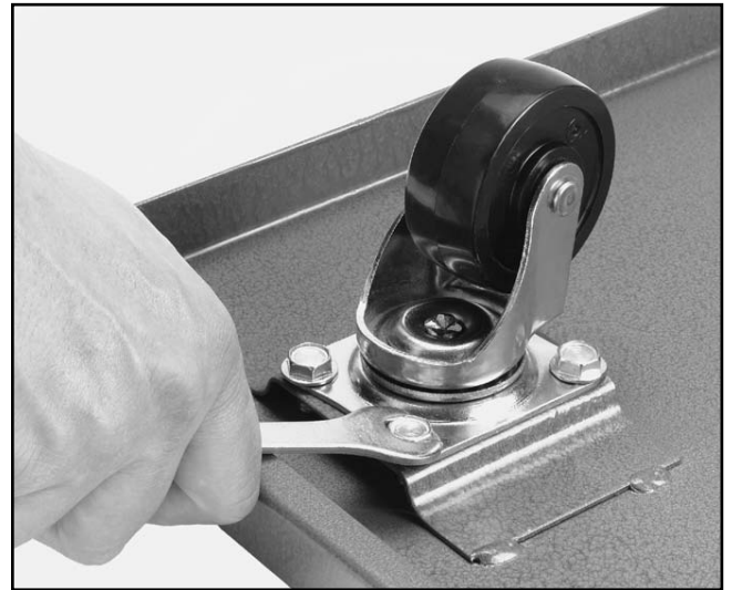
Figure 2. Mounting casters to base.
